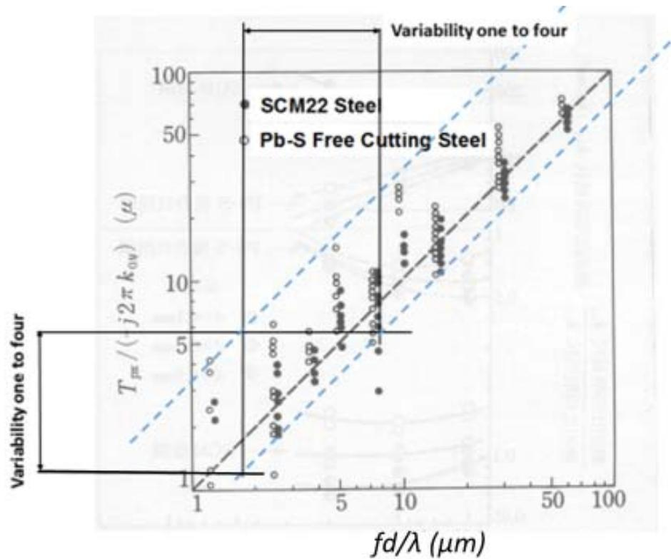
Fig.3 Experimental value of imaginary part effect of inner modulation measured in turning test.  $K_{ov}=Ft/bh, f=h, d=b$  [Hoshi 5), 6)]
