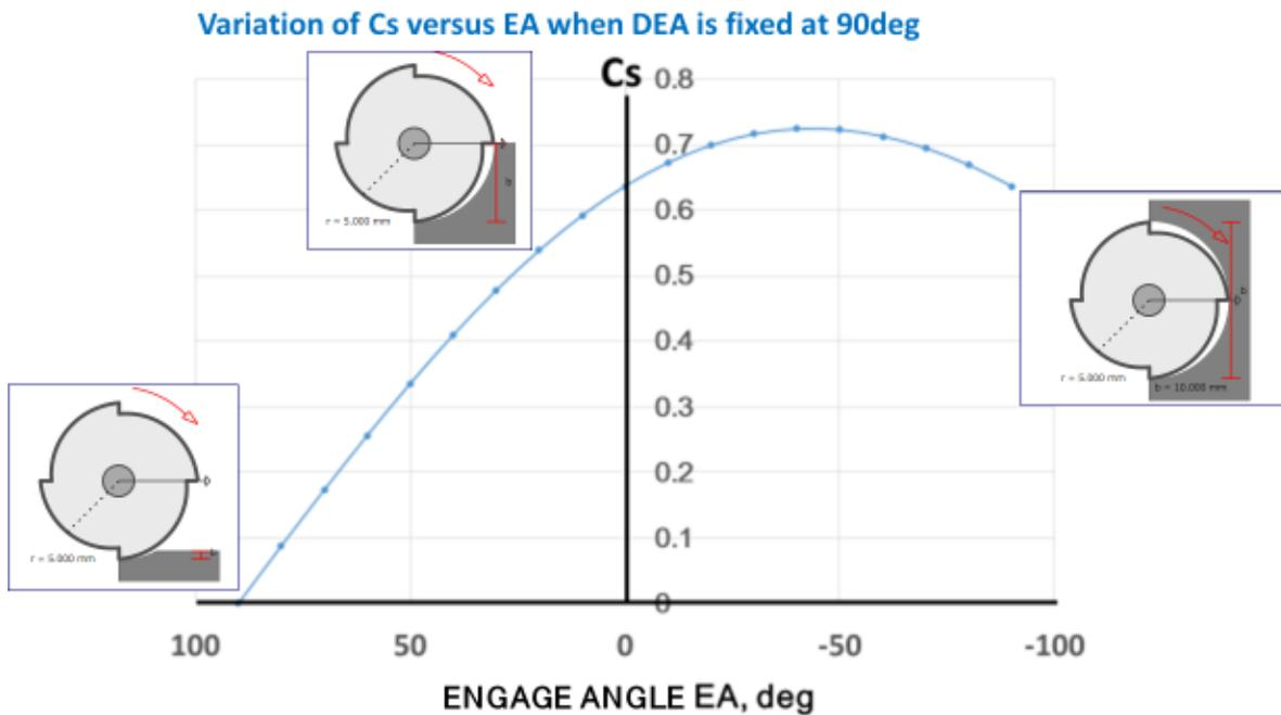
Fig.7 Variation of  $C_s$  for engage angle  $EA=-90$  to  $+90$ deg when disengage angle  $DA$  is fixed at 90deg
