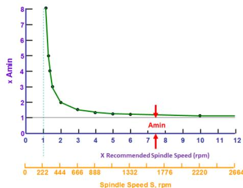
Fig. 8 Profile of low speed stability.
