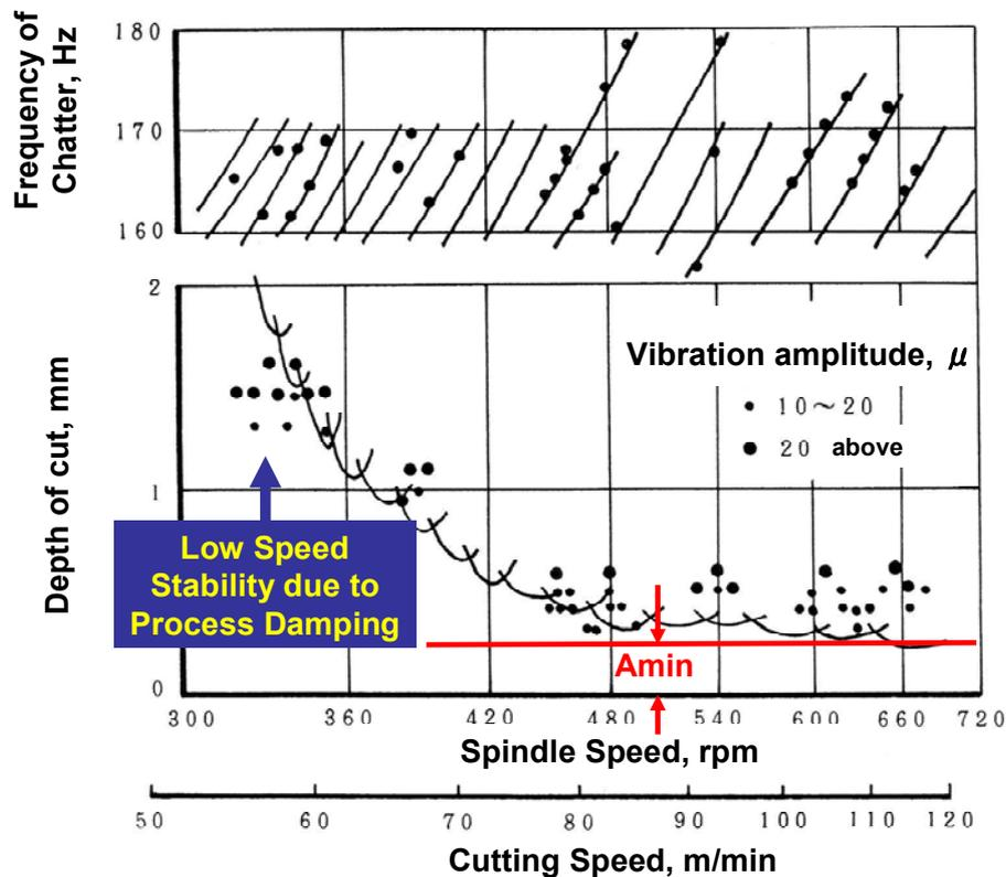
**Fig. 1** Experimental result of stability border diagram measured in turning test. (Lines represent results of computational simulation)
