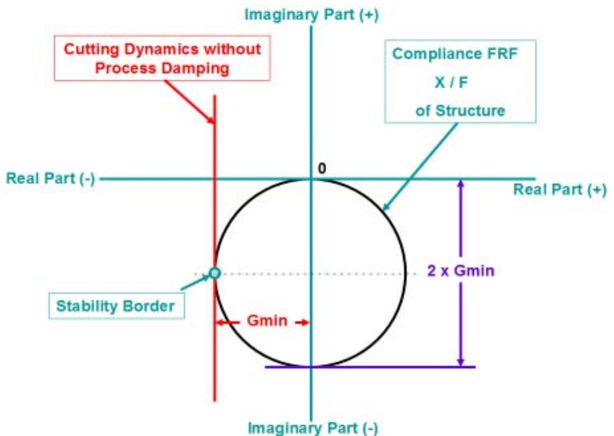
**Fig.4 Conventional stability border model in compliance vector diagram.**
