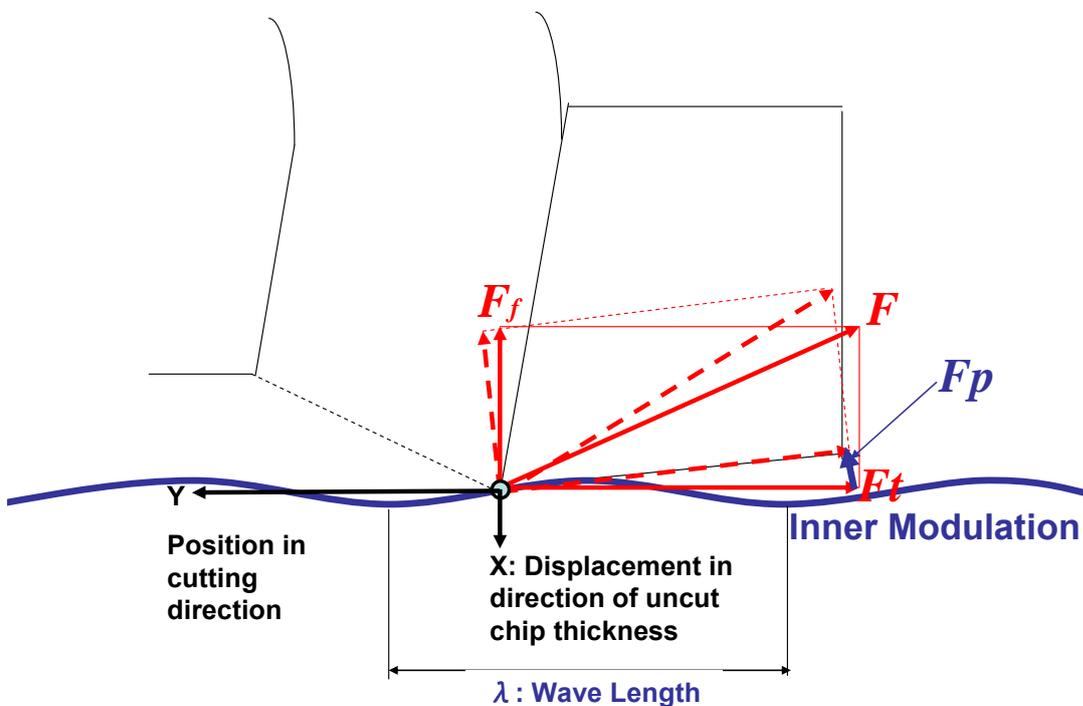
**Fig. 2 Hypothesis of Process Damping after Das and Tobias.**
