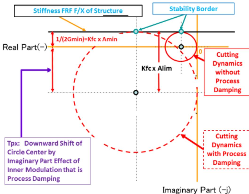
**Fig. 5 Stability border model in stiffness vector diagram.**
